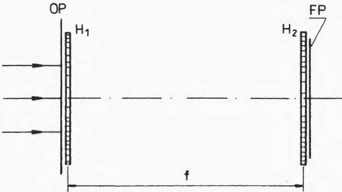
Fig. 3. Double holographic lens transformer ( $H_1, H_2$ ). Object plane OP is placed in the  $(x_o, y_o)$  and the Fourier plane FP — in the  $(x_f, y_f)$  planes of the coordinate system
