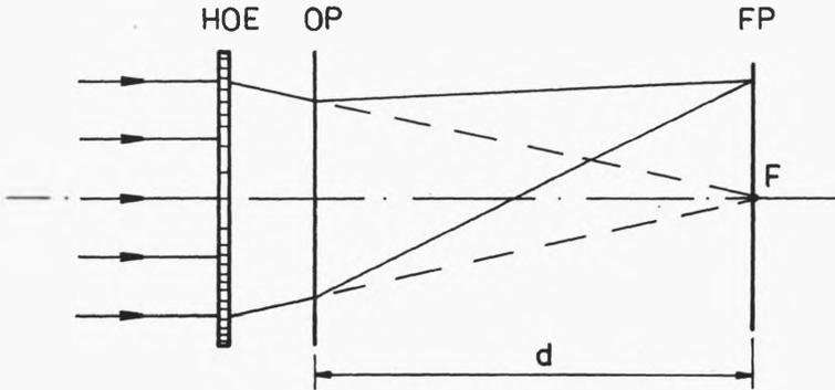
Fig. 4. Converging beam setup for Fourier transform
