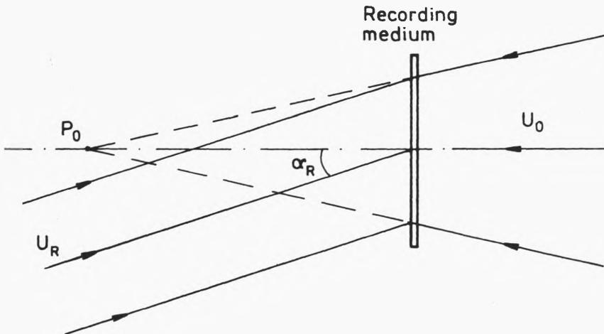
Fig. 1. Recording of an off-axis reflecting holographic element:  $\alpha$  is an offset angle,  $U_O$ ,  $U_R$  are the complex amplitudes of the object and reference point sources, respectively
