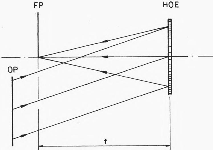
Fig. 2. Holographic reflecting element (HOE) as a Fourier transformer:  $f$  – focal length, OP – object plane, FP – Fourier plane
