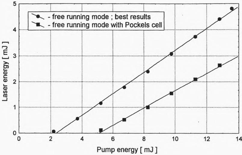
Fig. 2. Energy of free running mode (pump duration 200  $\mu$ s) vs. energy of pump incident on the slab:  $\bullet$  – best results for cavity without Pockels cell, with OC transmission 8%,  $\blacksquare$  – results for cavity with Pockels cell and 20% transmission of output coupler
