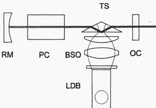
Fig. 1. Scheme of triangle slab laser: TS — Nd:YAG Brewster cut triangle slab, PC —  $LiNbO_3$  Pockels cell, OC — flat output coupler, RM — rear mirror with 2.5 m radius of curvature, BSO — beam shaping optics, LDB — quasi-cw laser diode bar SDL 3251-A1
