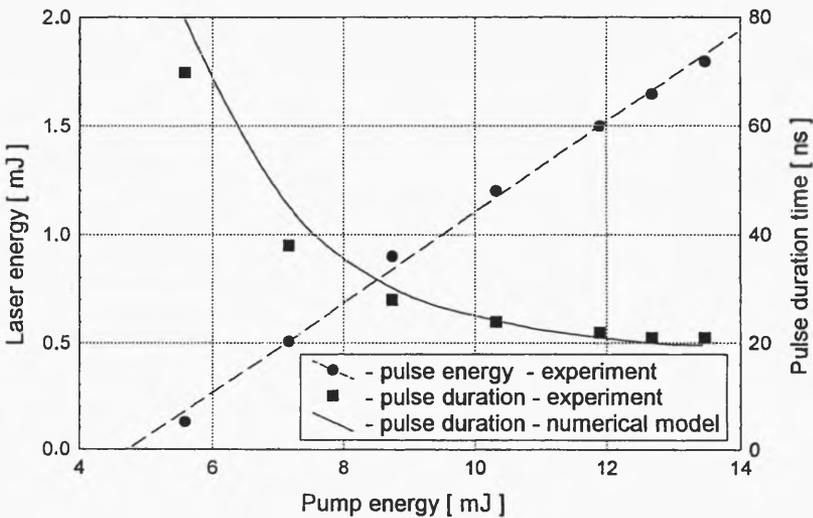
Fig. 4. Energy of Q-switched pulses and pulse durations as a function of pump energy: ● — energy of Q-switched pulses — experiment, ■ — pulse duration — experiment, solid curve — results of numerical simulation of pulse durations
