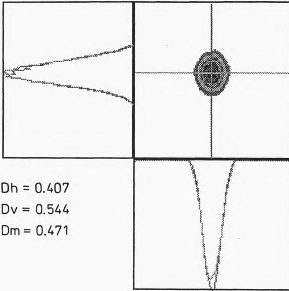
Fig. 5. Intensity distribution of output beam in focal plane of a lens of 300 mm focal length; correlation to Gaussian shape 0.94, averaged diameter 0.47 mm, averaged parameter  $M^2 < 1.15$
