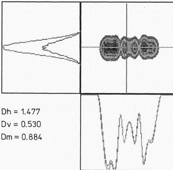
Fig. 3. Intensity distribution of output  $TEM_{0N}$  beam in focal plane of a lens of 300 mm focal length; estimated parameters  $M^2 \sim 1.2 \times 3.2$
