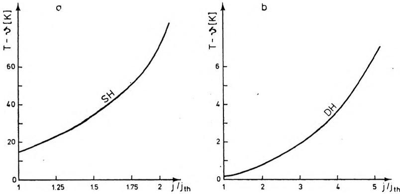
Fig. The graph of the changes in  $T - \Delta$  (that means of an error of the temperature estimation when the dependence of the thermal conduction coefficient on the temperature is neglected) vs. the feeding current density  $j$ :
