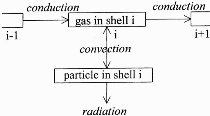
Fig. 2. Streams of heat energy in a shell
