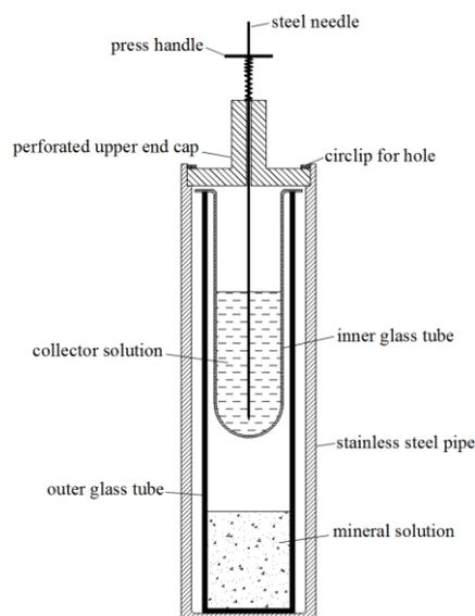
Fig. 2. Schematic diagram of the measuring cell
