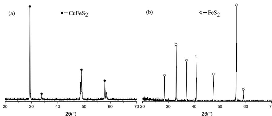
Fig. 1. XRD spectra of chalcopyrite and pyrite
