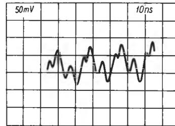
Fig. 4. Detector response to self-mode-locked  $\text{CO}_2$  TEA laser pulse
