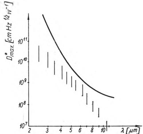
Fig. 2. Detectivity limit as a function of wavelength for PC (Cd,Hg)Te detectors
