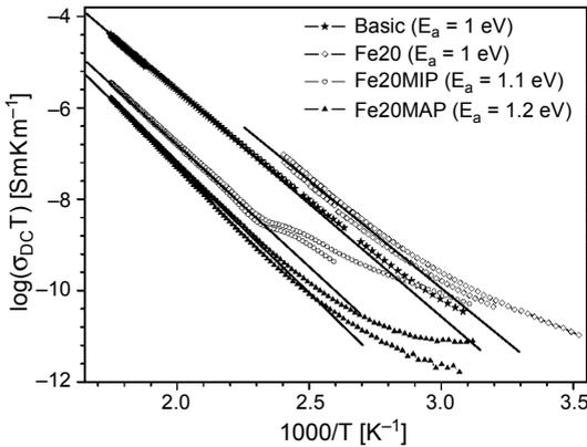
Fig. 3. Temperature dependences of  $(\sigma_{DC}T) = f(1/T)$  in Arrhenius coordinates on heating (upper set of symbols) and on cooling (lower set of symbols) for the basic SBS, Fe20, Fe20MIP and Fe20MAP glasses and their approximations by Arrhenius law – solid lines.
