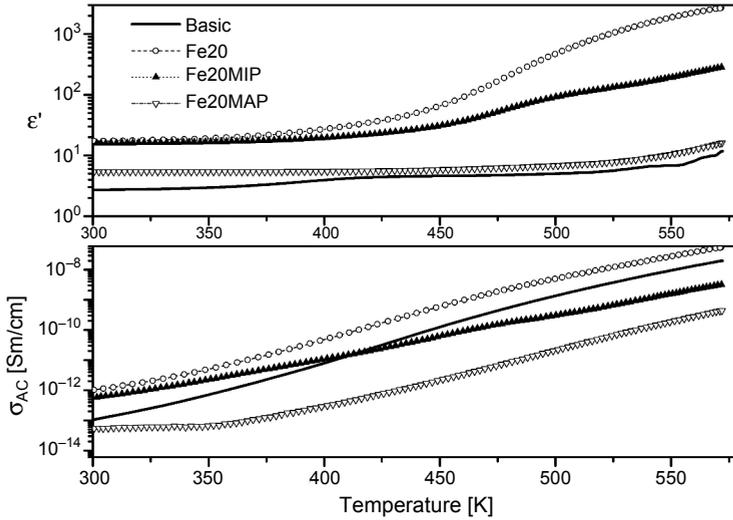
Fig. 2. Temperature dependences of dielectric permittivity  $\varepsilon'$  and conductivity  $\sigma_{AC}$  for microporous (Fe20MIP), macroporous (Fe20MAP) magnetic glasses, for two-phase Fe20 glass and basic (nonporous) alkali borosilicate glass at 5 Hz.
