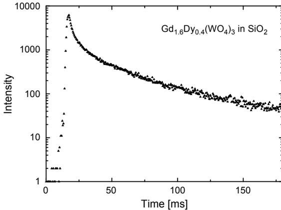
Fig. 3. Luminescence decays for material consisting of silica xerogel doped with  $\text{Gd}_{1.6}\text{Dy}_{0.4}(\text{WO}_4)_3$ . Observation wavelength at  $\lambda_{\text{obs}} = 575 \text{ nm}$ ; excitation wavelength  $\lambda_{\text{exc}} = 240 \text{ nm}$ .
