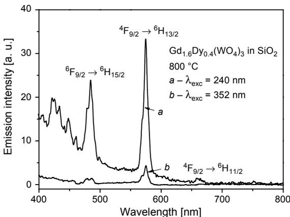
Fig. 2. Emission spectra of material consisting of silica xerogel doped with  $Gd_{1.6}Dy_{0.4}(WO_4)_3$ .
