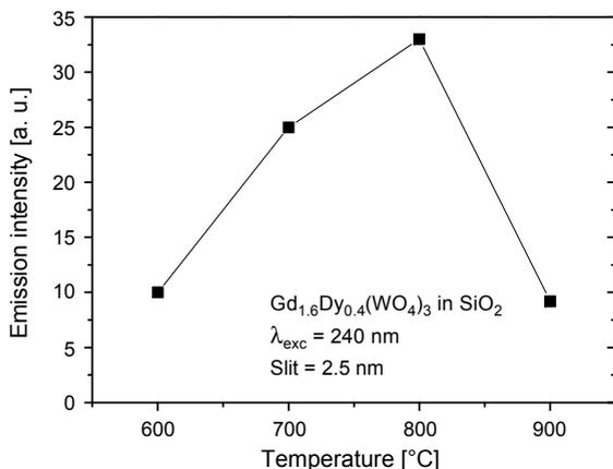
Fig. 4. The dependence of  $\text{Dy}^{3+}$  emission intensity  $I$  of the band  ${}^4F_{9/2} \rightarrow {}^6H_{13/2}$  at 575 nm with annealing temperature for material consisting of silica xerogel doped with  $\text{Gd}_{1.6}\text{Dy}_{0.4}(\text{WO}_4)_3$ . The lines are drawn as guide to the eyes.
