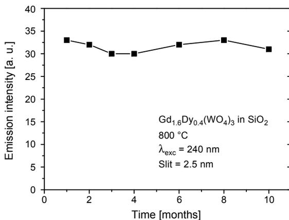
Fig. 5. The dependence of  $\text{Dy}^{3+}$  emission intensity  $I$  of the band  ${}^4F_{9/2} \rightarrow {}^6H_{13/2}$  at 575 nm with time for material consisting of silica xerogel doped with  $\text{Gd}_{1.6}\text{Dy}_{0.4}(\text{WO}_4)_3$ . The lines are drawn as guide to the eyes.
