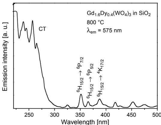
Fig. 1. Excitation spectra of material consisting of silica xerogel doped with  $\text{Gd}_{1.6}\text{Dy}_{0.4}(\text{WO}_4)_3$ .
