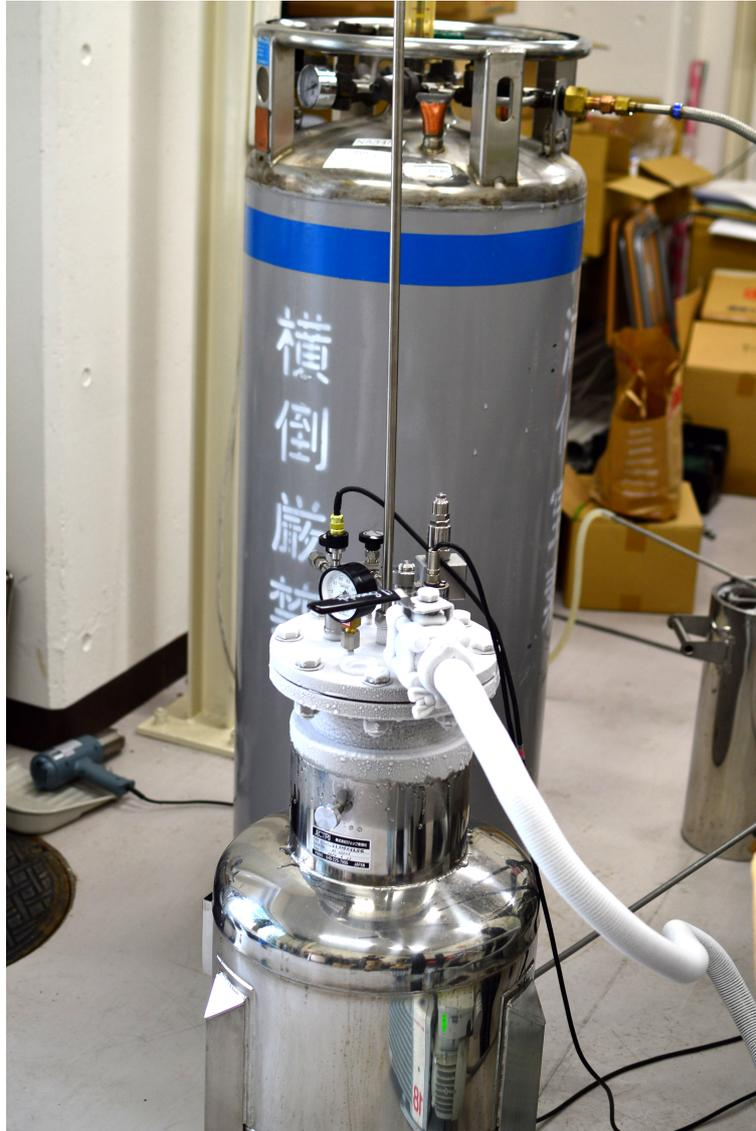
Figure 3.2 A detailed view on pressurized dewars. Small one is design for providing subcooled LN<sub>2</sub>.
