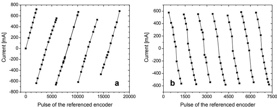
Fig. 5. Static measurement results of multiperiod (a), dynamic measurement results of multiperiod (b).
