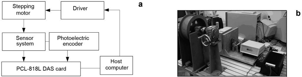
Fig. 4. Schematic of the experimental system (a), entity of the sensor and the experimental system (b).
