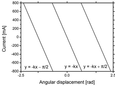
Fig. 3. Current/displacement curve of the sensor.
