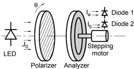
Fig. 6. Scheme of servo comparison displacement sensor.
