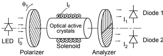
Fig. 2. Scheme of displacement-current comparator.
