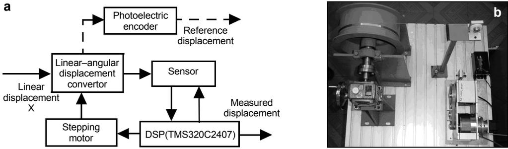
Fig. 7. Schematic diagram of the sensor and the test system (a), entity of the sensor and the test system (b).
