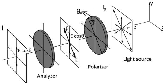
Fig. 1. Typical polarized light detecting system.
