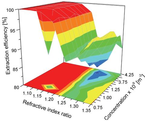
Fig. 5. 2D mapping of refractive index ratio and concentration. A strong dependence of refractive index ratio on light extraction efficiency. Radius of the scatter  $r = 1 \mu\text{m}$ .
