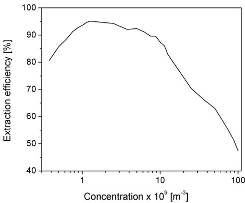
Fig. 4. Light extraction efficiency versus concentration of a scattering film. Radius of the scatter  $r = 1 \mu\text{m}$  and  $m = 1.55$ .
