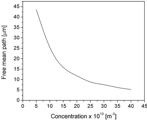
Fig. 3. Free-mean path of the photon versus the concentration. Radius of the scatter  $r = 1 \mu\text{m}$  and  $m = 1.55$ .
