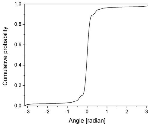
Fig. 2. Cumulative probability versus angle in radian for light scattering of a single particle of radius  $1 \mu\text{m}$ . The computer selects randomly a value between 0 and 1 and the scattered angle can be easily found. Note small scattered angle is preferred.
