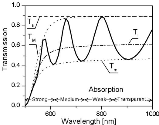
Fig. 2. Simulated transmission spectra (solid line) of a-Si:H and a clean substrate  $T_s$ . The film thickness of 600 nm,  $n_s$  of 1.6, and the same  $n(\lambda)$  and  $\alpha(\lambda)$  as in Ref. [10] are assumed. The envelopes  $T_M$ ,  $T_m$  and the smooth curve  $T_i$  are constructed from polynomial equations, respectively.
