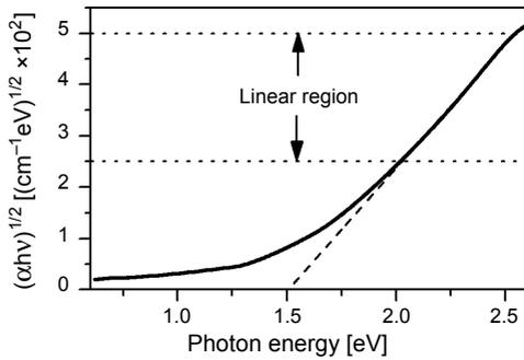
Fig. 8. A plot of  $(\alpha h\nu)^{1/2}$  versus the incident photon energy  $h\nu$  of a-GaP film.
