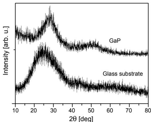
Fig. 3. XRD patterns of pulsed-dc sputtering deposited a-GaP film and the glass substrate.
