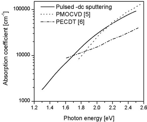
Fig. 6. Absorption coefficient of sputtered a-GaP film compared to that of a-GaP films from MOCVD and PECVD methods.
