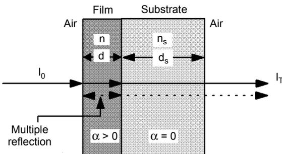
Fig. 1. Schematic diagram of light transmission through a film/substrate system.  $I_0$  is the intensity of the normal incident beam.  $I_T$  is the total intensity of transmitted beams, which is the superposition of the directly transmitted beams (solid line) and the beams transmitted after undergoing multiple reflections at the air/film and film/substrate interfaces (dashed line). In this model, transmittance is defined as  $T = I_T/I_0$ .
