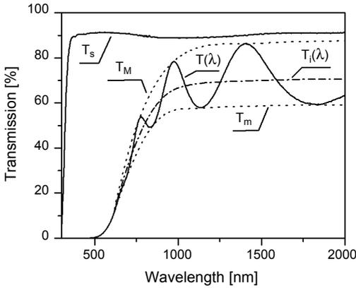
Fig. 4. Optical transmission spectra of a clean glass substrate,  $T_s$ , and that of the pulsed-dc sputtering a-GaP thin film on the substrate,  $T(\lambda)$ .  $T_M$ ,  $T_m$  are constructed envelopes for maxima and minima and  $T_i(\lambda)$  is a smooth curve evaluated from  $T_M$ ,  $T_m$ .
