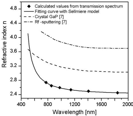
Fig. 5. The refractive index of the pulsed-dc sputtering deposited a-GaP film compared to those of a-GaP film deposited by rf-sputtering and crystalline GaP [7]. The dots are the values calculated from the transmission spectrum. The solid line is the fitted curve using Sellmeier equation expressed by:  $n(\lambda) = \sqrt{2.102 + 3.689\lambda^2 / (\lambda^2 - 432^2)}$ .
