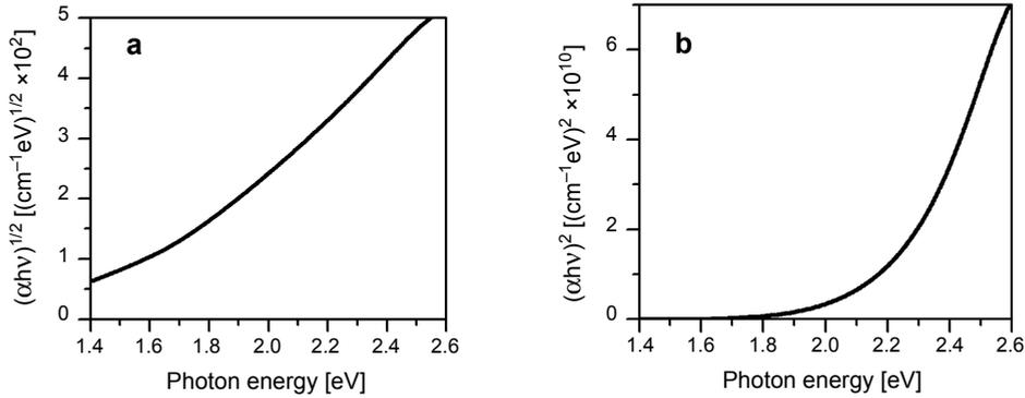
Fig. 7. Plots of  $(\alpha h\nu)^{1/2}$  vs.  $h\nu$  (a) and  $(\alpha h\nu)^2$  vs.  $h\nu$  (b) of the pulsed-dc sputtering a-GaP.
