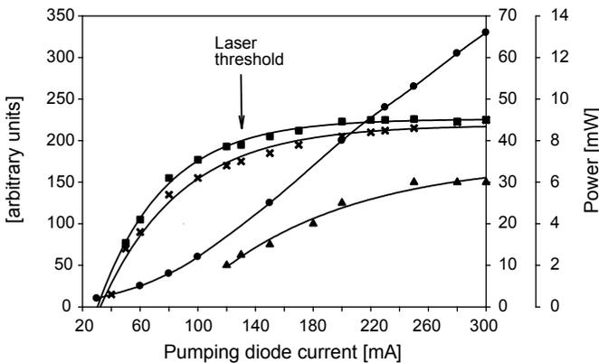
Fig. 2. Results of measurements: filled circle – 971 nm pumping power measured at the end of the fiber (right-hand scale from 10 to 70 mW); filled triangle – laser output power at 545 nm (right-hand scale, from 2 to 6 mW); cross – side fluorescence at 545 nm, with no output mirror in place (left-hand scale, from 0 to 300, arbitrary units); filled square – side fluorescence at 545 nm, with output mirror in place (left-hand scale, from 0 to 300, arbitrary units).
