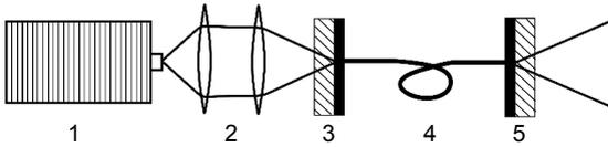
Fig. 1. Experimental arrangement: 1 – pumping diode (971 nm), emission area  $1\ \mu\text{m}\times 5\ \mu\text{m}$ , power 300 mW max output; 2 – double lens focusing system; 3 – dichroic mirror, 95% transmission at 971 nm and almost totally reflecting at 545 nm; 4 – ZBLAN:Er<sup>3+</sup> optical fiber, core diameter 1.7  $\mu\text{m}$ , length – 230 cm, Er<sup>3+</sup> concentration – 100 ppm; 5 – dichroic mirror, 41% transmission at 545 nm, totally reflecting at 971 nm.
