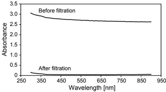
Fig. 9. Absorbance of water suspension of calcium carbonate before and after filtration in the pre-concentrator.
