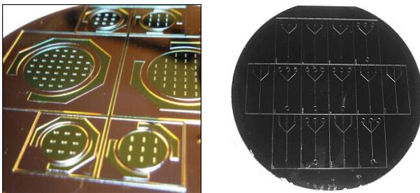
Fig. 4. Masters of a pre-concentrator and microfluidic chip, with negative patterns of microchannels made in UV-curable epoxy resin SU-8.
