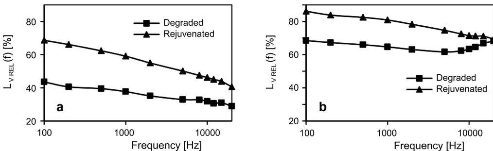
Fig. 6. Luminance of set B (a) and set C (b) samples, relative to luminance of set A, as a function of frequency, for a 100 V square-wave excitation.
