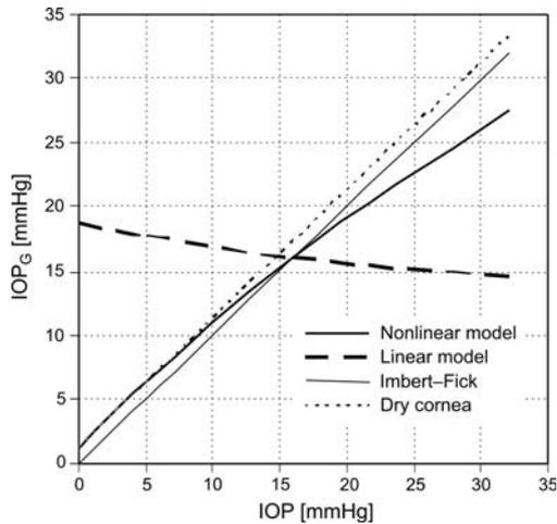
Fig. 4. Calculated  $IOP_G$  for model made of: linear-elastic material and nonlinear-elastic material, depending on IOP. Grey lines represent Goldmann idealization: broken line – pressure measured on dry (not wetted with lacrimal fluid) cornea, solid line expresses Imbert–Fick law (Eq. (1)) and so takes into account the influence of surface tension in lacrimal film. All bold lines satisfy condition  $IOP_G = IOP = 16$  mmHg (nominal).
