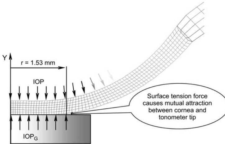
Fig. 3. Cross-section of cornea.  $Y$ -axis is symmetry axis. Surface tension force reduces resultant  $IOP_G$  force needed to flatten corneal apex over radius  $r = 1.53$  mm. Forces originating from IOP and from reaction of part of cornea surrounding disc act from inside on flattened disc.
