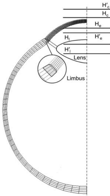
Fig. 1. Schematic finite element model of the eyeball with principal planes of the eye optical system.
