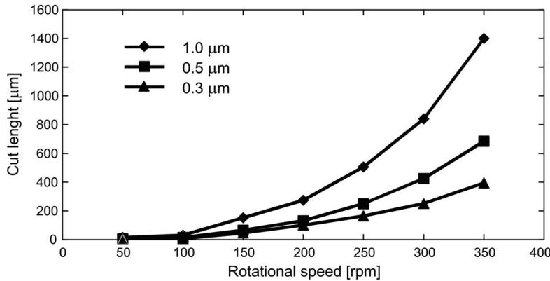
Fig. 1. Graph of cut off length vs. rotational speed using sandpaper of size 1.0 μm, 0.5 μm and 0.3 μm. The equation of the curve  $y = 0.0041x^2 - 0.3352x$ .
