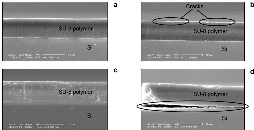
Fig. 3. Waveguide surface for set 1 (a), set 2 (b), set 3 (c), and set 4 (d).
