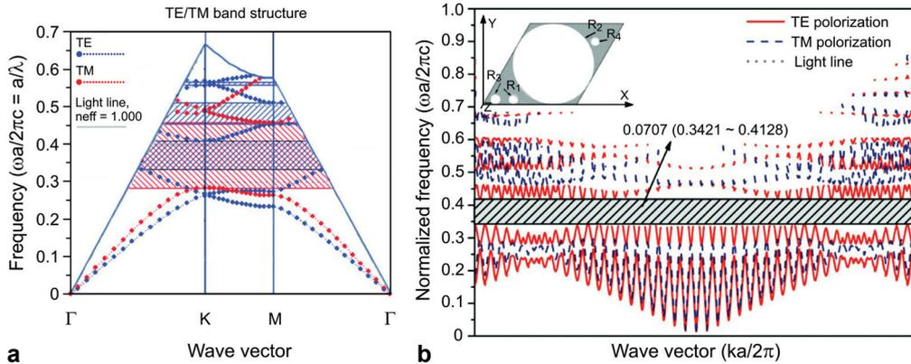
Fig. 5. The optimized structure with four circular holes in its unit cell and the corresponding band diagram for TM mode (solid lines) and TE mode (dotted lines);  $\Gamma$ ,  $K$ , and  $M$  refer to the corner points of the 1/8 Brillouin zone – **a**. The optimized structure with four circular holes in its unit cell and the corresponding band diagram for TE and TM polarizations of full zone – **b**.
