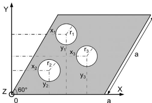
Fig. 1. The unit cell of a 2D PC with hexagonal lattice composed of three circular holes in silicon substrate.
