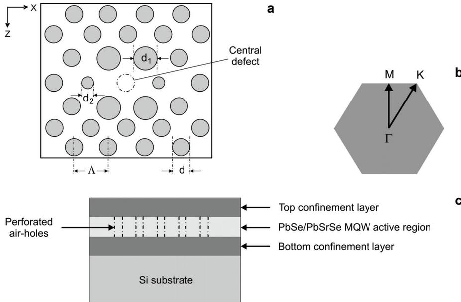
Fig. 1. Top view of triangular photonic crystal lattice structure (a). Schematic of the first Brillouin zone for the hexagonal lattice pattern (b). Schematic view of the MBE-grown sample with photonic crystal structure in the active region (c).
