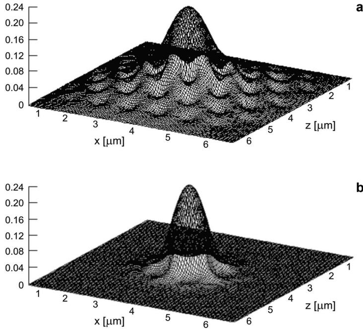
Fig. 4. Resonating electric field distribution at  $\lambda = 4.17 \mu\text{m}$  for multi-modal (a), and single modal (b) conditions.
