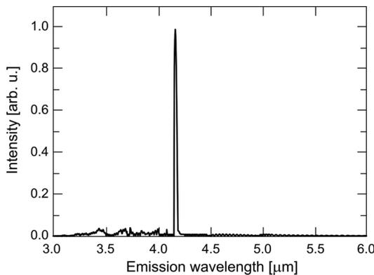
Fig. 5. Spectral response from DFT calculations after FDTD analysis of the resonating defect cavity.
