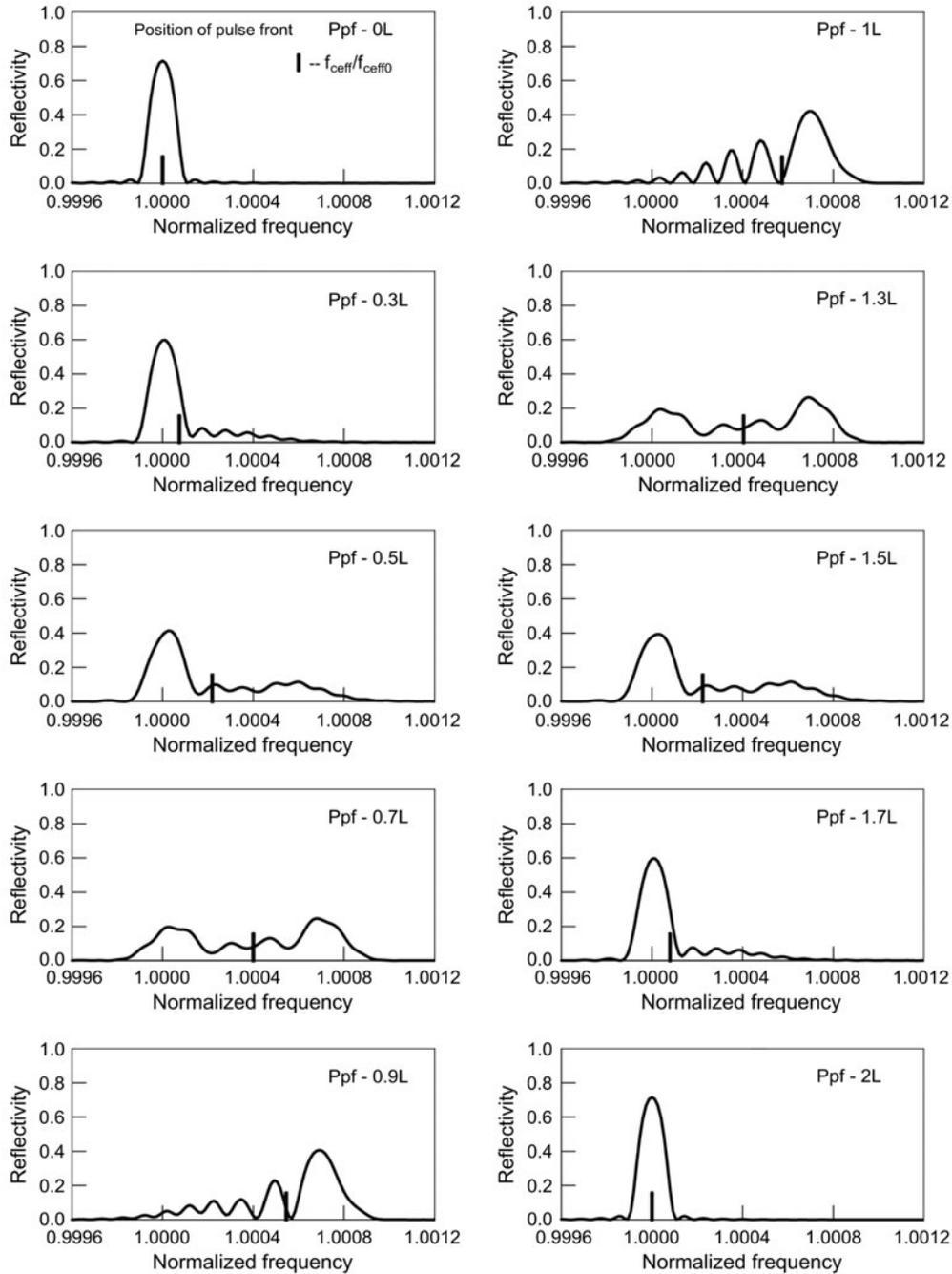
Fig. 2. The reflected spectrum and the corresponding effective central frequency of the apodized grating subjected to the single half-sine compressive strain pulse with an amplitude of  $A = 1000 \mu\epsilon$  and a rise length of  $b = L/2$ , for the different position of the pulse front with respect to the beginning of the grating.
