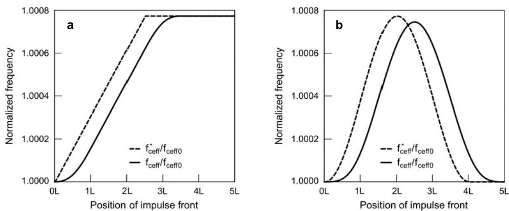
Fig. 3. The normalized effective central frequency of the apodized gratings: non-distorting one (dashed line) and distorting one (solid line), as a function of the front position of the acting compressive strain pulses. These pulses have an amplitude of  $A = 1000 \mu\varepsilon$  and the shapes: constant slope front step function with a rise length of  $b = 2.5L$  (a), single whole-sine with a rise length of  $b = 2.0L$  (b).
