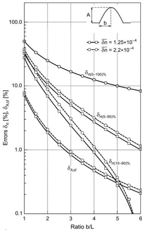
▲ Fig. 4. The converting errors of the apodized gratings as functions of the ratio  $b/L$ , for the half-sinusoidal strain pulse.
