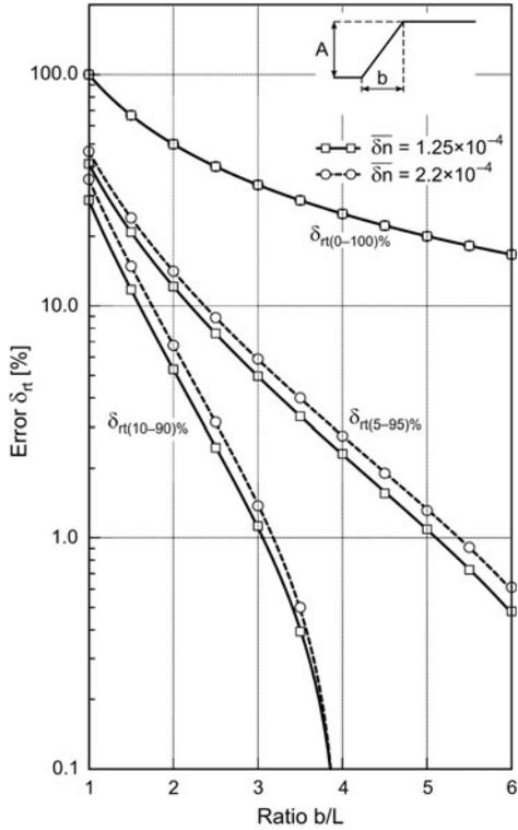
Fig. 6. The rise-time error of the apodized gratings as functions of the ratio  $b/L$ , for the constant slope front step function.
