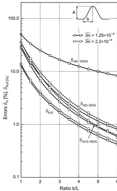
Fig. 5. The converting errors of the apodized gratings as functions of the ratio  $b/L$ , for the whole-sinusoidal strain pulse.
