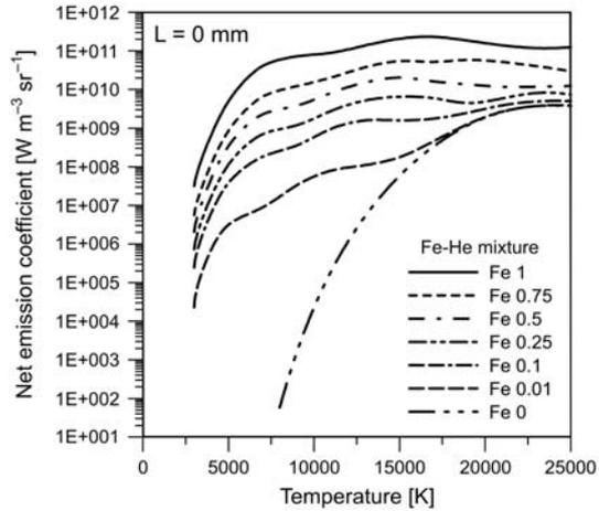
Fig. 3. Net emission coefficient of iron-helium plasma for different mass fractions of iron. Optically thin plasma  $L = 0$ . Total pressure 0.1 MPa.
