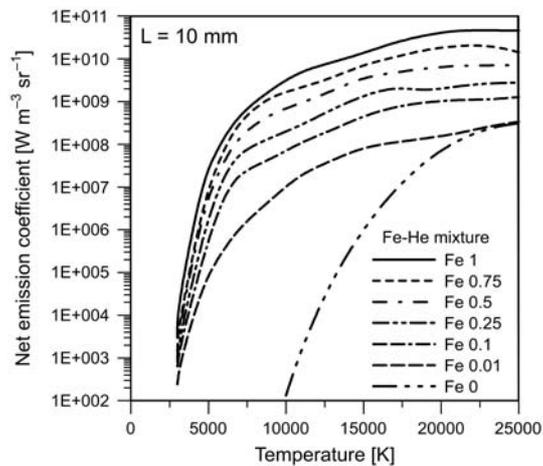
Fig. 5. Net emission coefficient of thermal iron-helium plasma for different mass fractions of iron. Plane layer 10 mm thick. Total pressure 0.1 MPa.
