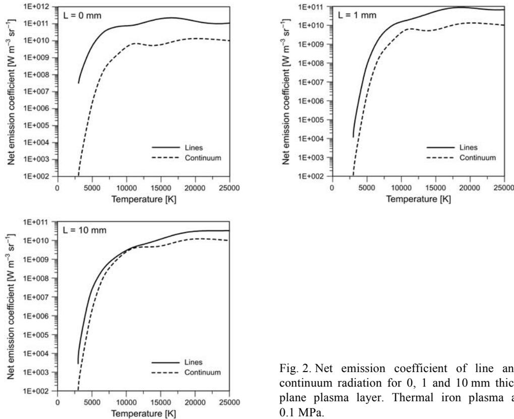
Fig. 2. Net emission coefficient of line and continuum radiation for 0, 1 and 10 mm thick plane plasma layer. Thermal iron plasma at 0.1 MPa.
