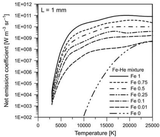
Fig. 4. Net emission coefficient of iron-helium plasma for different mass fractions of iron. Plane layer 1 mm thick. Total pressure 0.1 MPa.
