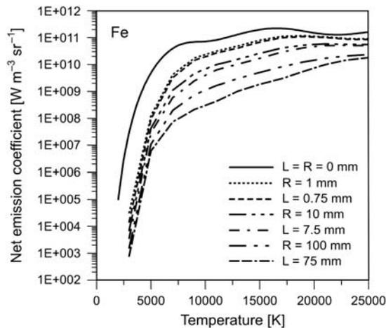
Fig. 6. Net emission coefficients for spherical plasma and plane plasma layer. Pure iron, pressure 0.1 MPa.
