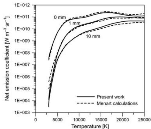
Fig. 1. Net emission coefficient of thermal iron plasma at 0.1 MPa. Solid lines show results obtained in the present work, the dashed lines show results from MENART and MALIK [5].
