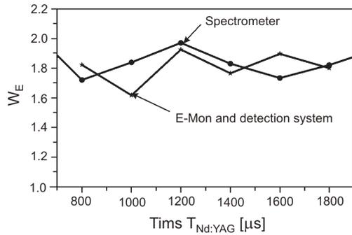
Fig. 12. Influence of the energy of Nd:YAG laser on the calibration factor. The maximum value of the laser energy is 500 mJ and it corresponds to the time value  $T_{\text{Nd:YAG}} = 1200 \mu\text{s}$  in the figure; the data are taken from the documentation provided by the laser producer.
