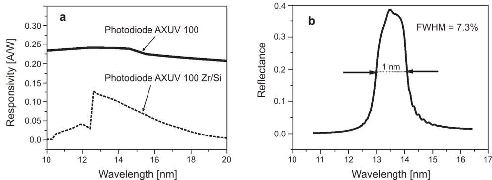
Fig. 1. Spectrum characteristic of photodiode responsivity (a) and multilayer reflectivity (b).
