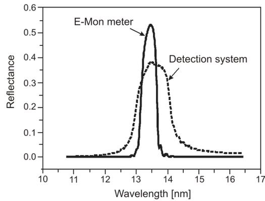
Fig. 6. Spectrum characteristics of mirrors reflectivity used in the detection system and E-Mon energy meter.
