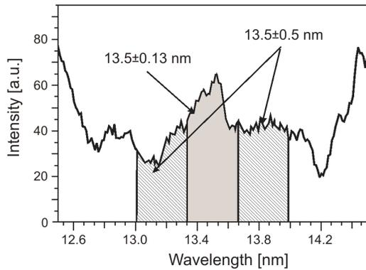
Fig. 3. Spectrum of radiation emitted by laser-plasma source with Xe/He gas puff target in two analyzed ranges of wavelengths.
