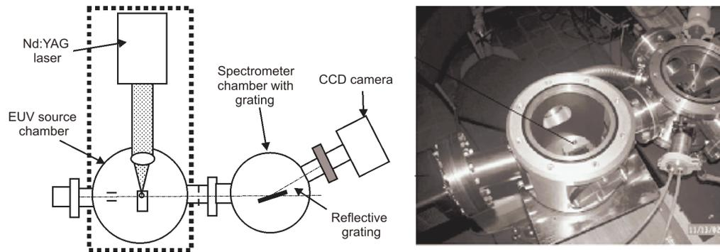
Fig. 7. Scheme and view of the spectrometer.
