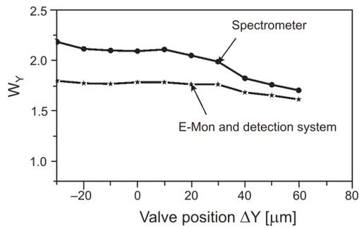
Fig. 10. Influence of the valve position relative to Nd:YAG laser beam on the calibration factor.
