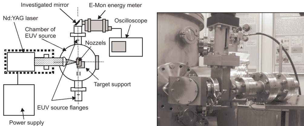
Fig. 5. Scheme and view of laboratory setup for measurements of the features of the system elements.
