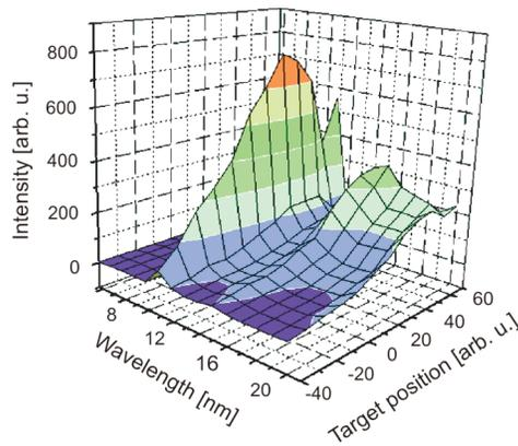
Fig. 4. Spectrum of radiation emitted by laser-plasma source for different positions of laser beam on target surface.
