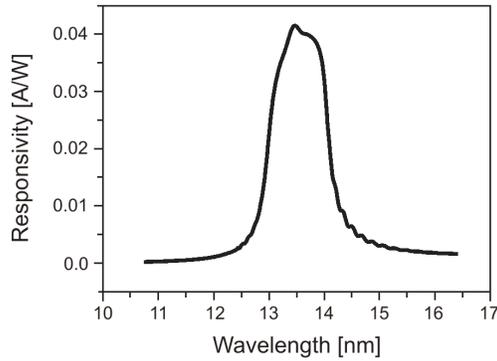
Fig. 2. Theoretical characteristic of the system responsivity determined by catalogue parameters of its elements.
