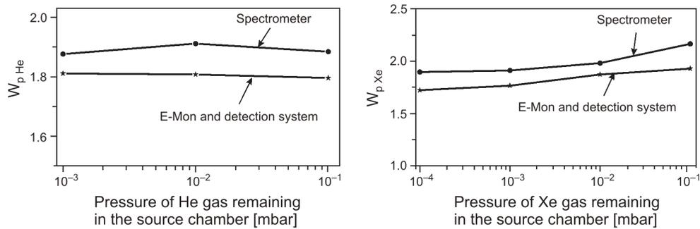
Fig. 11. Influence of pressure of the remaining gases in the source chamber on the calibration factor.
