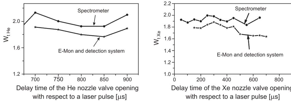
Fig. 8. Influence of delayed time of nozzle opening relative to Nd:YAG laser pulse on the calibration factor.
