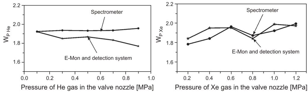
Fig. 9. Influence of the pressures of gases in the target nozzle on the calibration factor.
