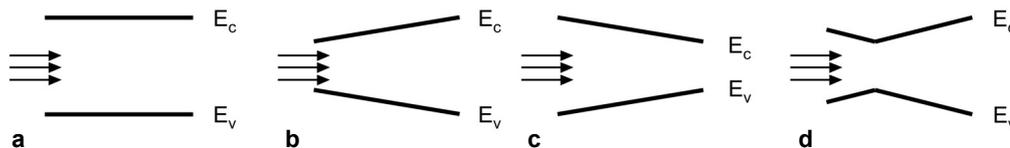
Fig. 2. Types of band-gap profiling: without profiling (a), normal (b), reverse (c), double (d) [11, 12].
