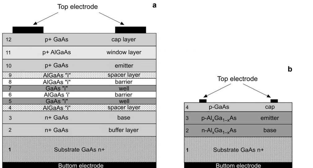
Fig. 1. Solar cell structure:  $p-i(\text{MQW})-n$  (a), graded solar cell (b).
