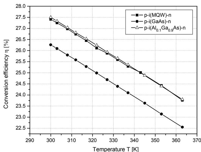
Fig. 4. Conversion efficiency of optimized MQW and reference solar cells vs. temperature.
