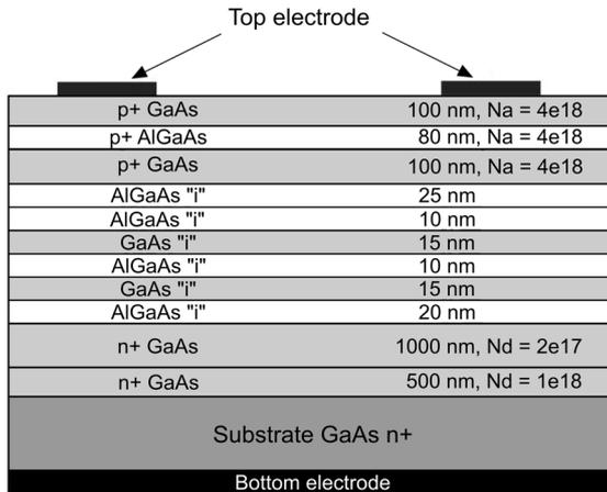
Fig. 3. Optimized structure of MQW solar cell.
