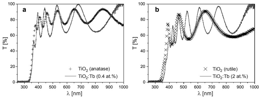
Fig. 3. Transmission spectra of: TiO<sub>2</sub>:Tb (0.4 at.% Tb) compared to TiO<sub>2</sub>-anatase (a) and TiO<sub>2</sub>:Tb (2 at.% Tb) compared to TiO<sub>2</sub>-rutile thin films on SiO<sub>2</sub> (b).
