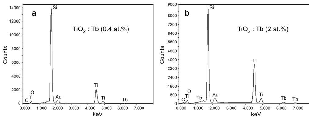
Fig. 1. EDS spectra of as-deposited  $\text{TiO}_2:\text{Tb}$  thin films on silicon: 0.4 at.% Tb (a) and 2 at.% Tb (b).
