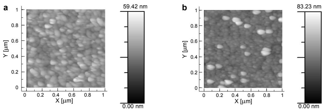
Fig. 2. AFM images of  $\text{TiO}_2:\text{Tb}$  thin films on  $\text{SiO}_2$ : 0.4 at.% Tb (a) and 2 at.% Tb (b).
