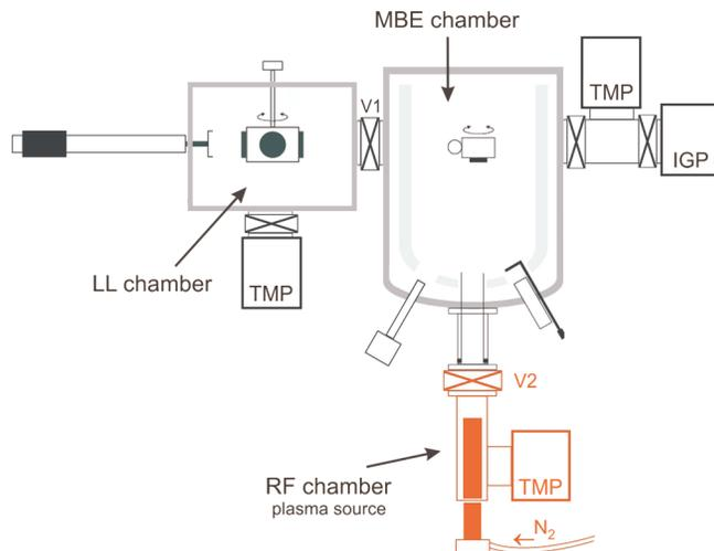
Fig. 1. Schematic cross-section of the RF MBE used for the growth of (In,Ga)(As,N)/GaAs DQW p-i-n photodetectors.
