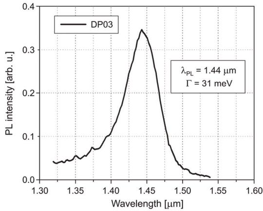
Fig. 2. PL spectra of #DP03 structure.
