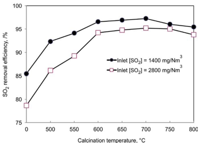
Fig. 4. Effect of calcination temperature on the SO<sub>2</sub> removal efficiency
