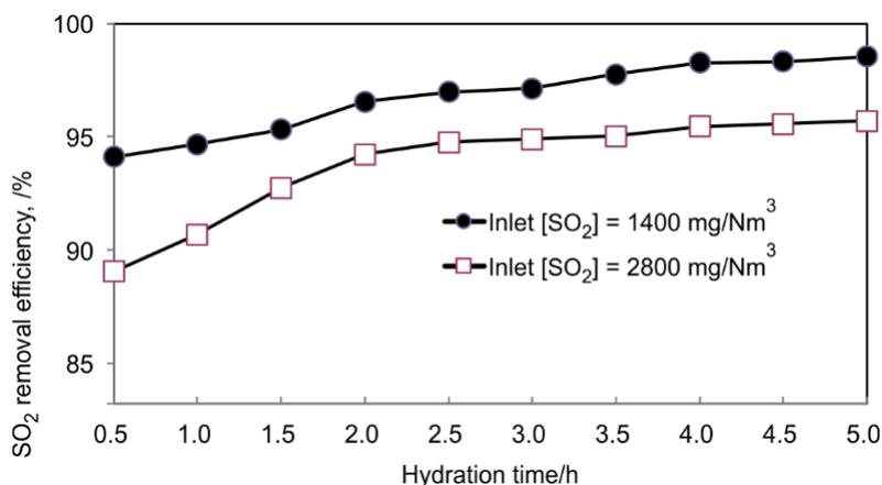
Fig. 5. Effect of hydration time on the SO<sub>2</sub> removal efficiency
