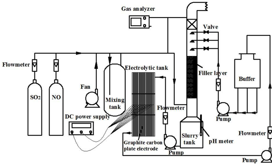
Fig. 3. Schematic diagram of the pilot-scale reactor
