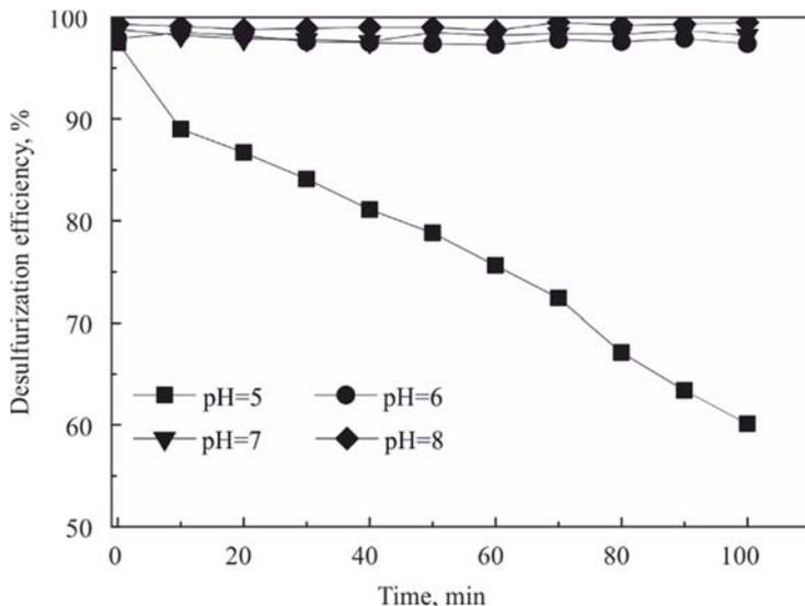
Fig. 10. Effect of pH on SO<sub>2</sub> removal efficiency (25 °C, concentrations of: Fe(II)EDTA – 0.05 mol·dm<sup>-3</sup>, NO<sub>x</sub> – 400 mg·m<sup>-3</sup>, SO<sub>2</sub> – 1400 mg·m<sup>-3</sup>, O<sub>2</sub> – 20%, 2.0 V, 15 A)
