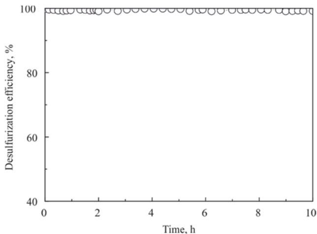
Fig. 18. Desulfurization efficiency in a pilot-scale reactor (25 °C, concentrations of: Fe(II)EDTA – 0.05 mol·dm<sup>-3</sup>, pH 5–6, O<sub>2</sub> – 18%, 2.1 V, 62 A)
