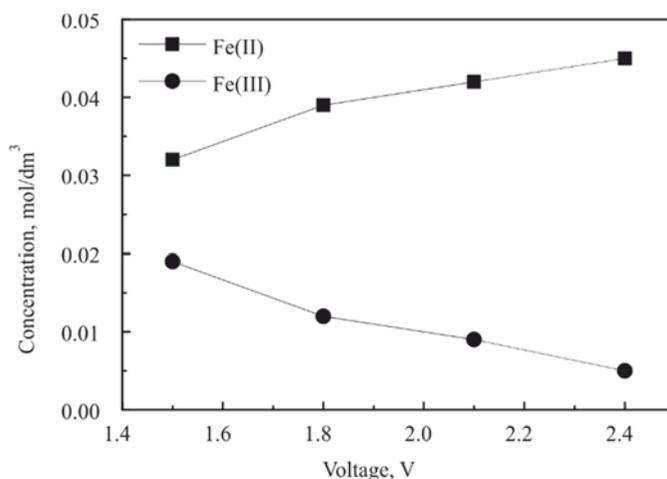
Fig. 14. Effect of voltage on Fe(II) and Fe(III) concentrations in ammonia-Fe(II)EDTA solution (25 °C, concentrations of: Fe(II)EDTA –  $0.05 \text{ mol}\cdot\text{dm}^{-3}$ , pH 5–6,  $\text{NO}_x$  –  $400 \text{ mg}\cdot\text{m}^{-3}$ ,  $\text{SO}_2$  –  $1400 \text{ mg}\cdot\text{m}^{-3}$ ,  $\text{O}_2$  – 20%)
