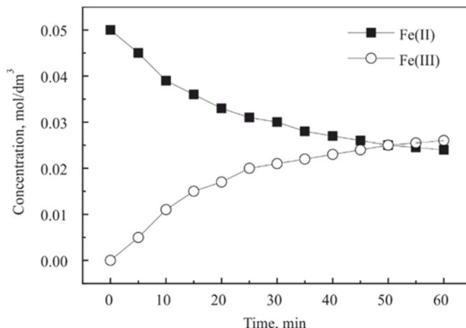
Fig. 7. Effect of reaction time on F(II) and Fe(III) concentrations in ammonia-Fe(II)EDTA (25 °C, pH 5–6, concentrations of: Fe(II)EDTA – 0.05 mol·dm<sup>-3</sup>, NO<sub>x</sub> – 400 mg·m<sup>-3</sup>, SO<sub>2</sub> – 1400 mg·m<sup>-3</sup>, O<sub>2</sub> – 20%)
