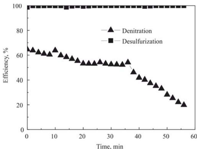
Fig. 6. Simultaneous removal of  $SO_2$  and  $NO_x$  with ammonia-Fe(II)EDTA (25 °C, pH 5–6, concentrations of: Fe(II)EDTA – 0.05 mol·dm<sup>-3</sup>,  $NO_x$  – 400 mg·m<sup>-3</sup>,  $SO_2$  – 1400 mg·m<sup>-3</sup>,  $O_2$  – 20%)
