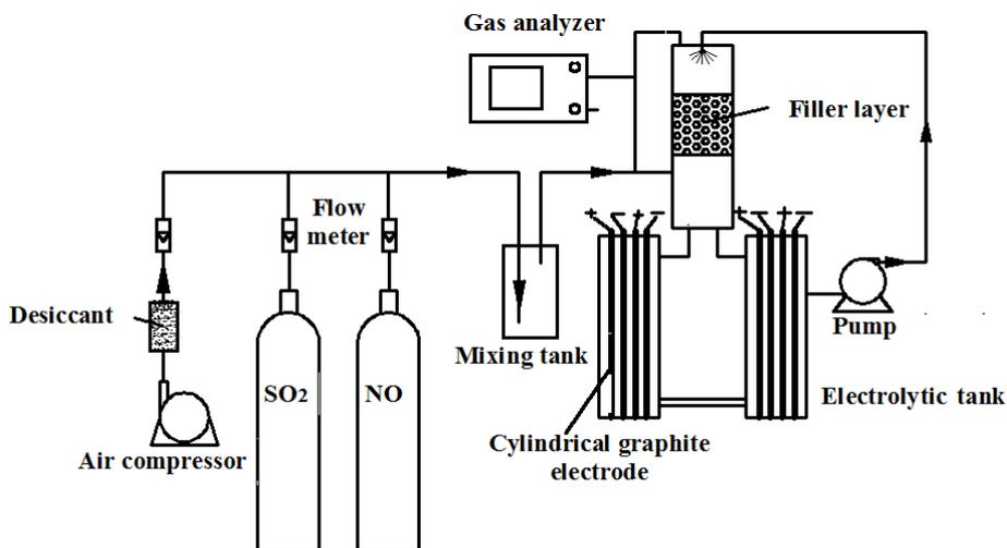
Fig. 1. Schematic diagram of the bench-scale reactor desiccant
