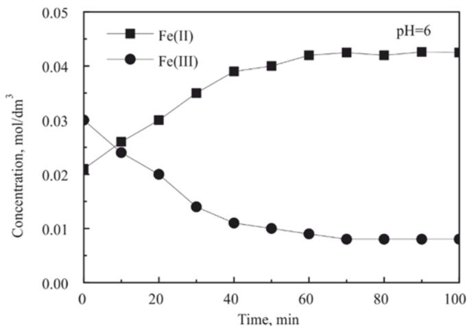
Fig. 9.  $\text{Fe(II)}$  and  $\text{Fe(III)}$  concentrations in ammonia- $\text{Fe(II)EDTA}$  solution during electrochemical regeneration (25 °C, pH 6, concentrations of:  $\text{Fe(II)EDTA} - 0.05 \text{ mol} \cdot \text{dm}^{-3}$ ,  $\text{NO}_x - 400 \text{ mg} \cdot \text{m}^{-3}$ ,  $\text{SO}_2 - 1400 \text{ mg} \cdot \text{m}^{-3}$ ,  $\text{O}_2 - 20\%$ , 2.0 V, 15 A)
