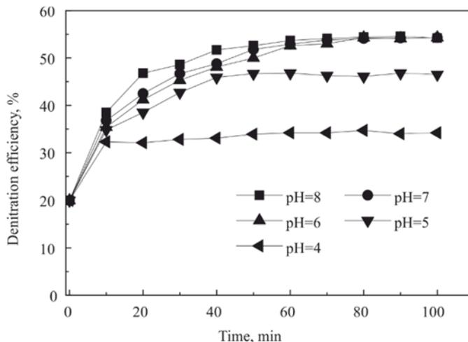
Fig. 8. Effect of pH on  $\text{NO}_x$  removal efficiency (25 °C, concentrations of:  $\text{Fe(II)EDTA} - 0.05 \text{ mol} \cdot \text{dm}^{-3}$ ,  $\text{NO}_x - 400 \text{ mg} \cdot \text{m}^{-3}$ ,  $\text{SO}_2 - 1400 \text{ mg} \cdot \text{m}^{-3}$ ,  $\text{O}_2 - 20\%$ , 2.0 V, 15 A)
