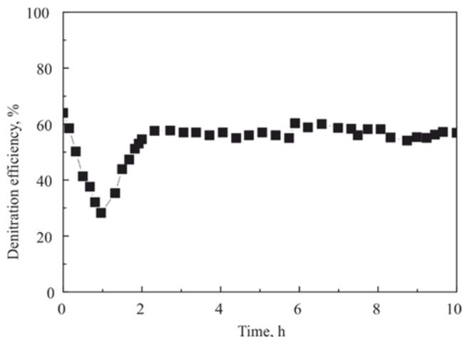
Fig. 16. Denitration efficiency in a pilot-scale reactor
