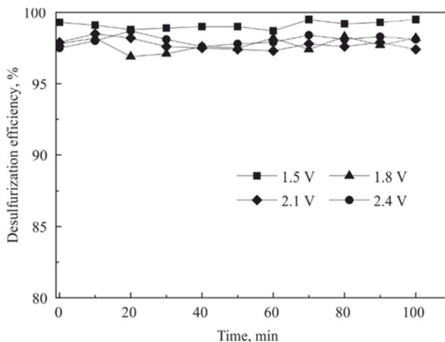
Fig. 15. Effect of voltage on  $\text{SO}_2$  removal efficiency (25 °C, concentrations of: Fe(II)EDTA –  $0.05 \text{ mol}\cdot\text{dm}^{-3}$ , pH 5–6,  $\text{NO}_x$  –  $400 \text{ mg}\cdot\text{m}^{-3}$ ,  $\text{SO}_2$  –  $1400 \text{ mg}\cdot\text{m}^{-3}$ ,  $\text{O}_2$  – 20%)
