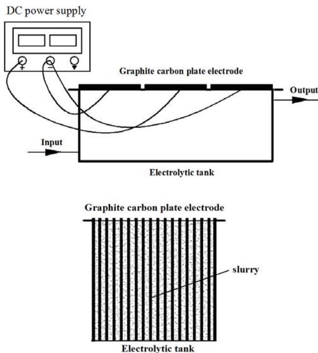
Fig. 5. Side-view of the graphite plate electrodes
