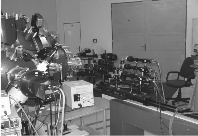
Fig. 6. View of the plasma chamber and interferometric registration system.
