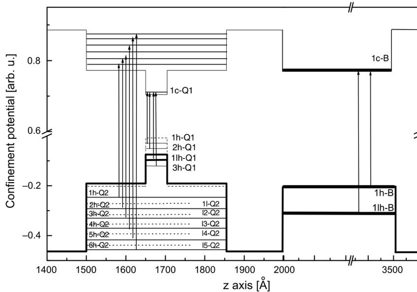
Fig. 3. Calculated confinement potential and energy levels obtained theoretically for three different quantum wells: for well defined quantum regime ( $L_z = 55$  Å), for quasi-quantum regime ( $L_z = 355$  Å), and for quasi-bulk regime ( $L_z = 1500$  Å).
