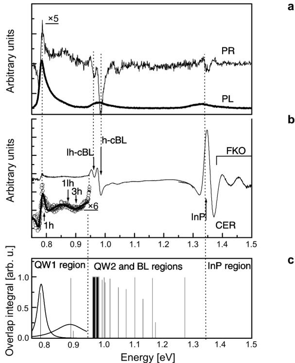
Fig. 2. Room temperature photoreflectance, luminescence (a), and electroreflectance spectra of InGaAsP QW structure (b); theoretical (vertical lines) and experimental (Lorentzian lines) optical transition intensities (c).
