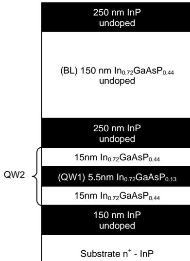
Fig. 1. Schematic structure of InGaAsP quantum well.
