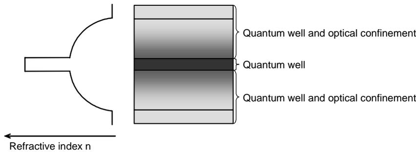
Fig. 3. Schematic GRINSH structure.
