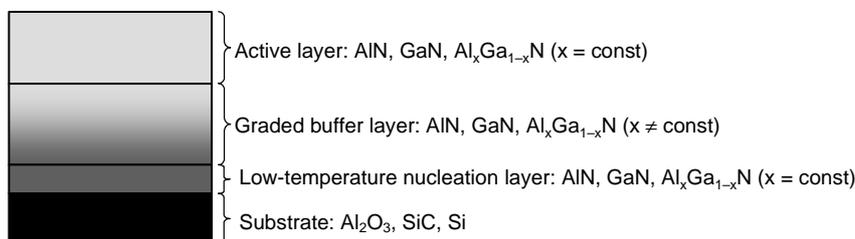
Fig. 2. Structure of heteroepitaxially grown A<sup>III</sup>N compounds with graded buffer layer.
