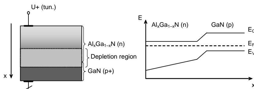
Fig. 5. Schematic structure of tunable photodetector.
