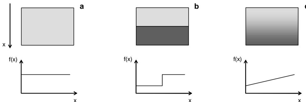
Fig. 1. Schematic representation of materials function in different structures; homogenous material (a), junction (b), FGM (c).
