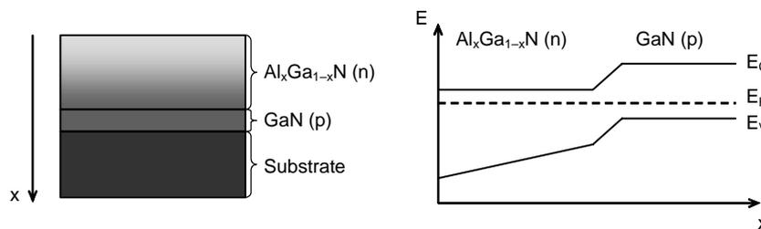
Fig. 4. Schematic structure of p-n photodiode with graded layer.
