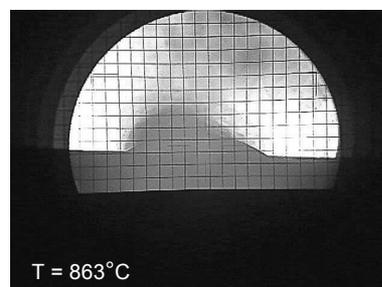
Fig. 4. Wetting of magnesium aluminosilicate substrate by Pb21K vitrified bond.
