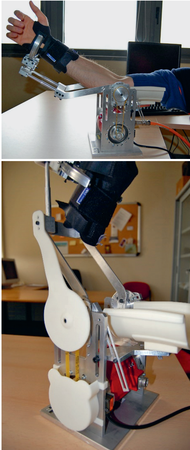
Fig. 4. Prototype of a symmetrical device with 2-side drive system: a) view of the device, b) view of 3D-printed ergonomic elements
